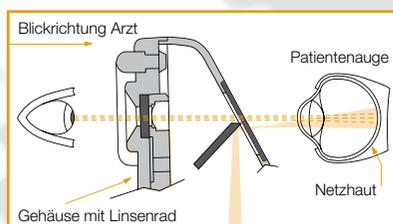
Reflexes from the cornea and iris are avoided by separating the observational and illuminating light beams (Gullstrand's principle). The illuminated retinal area is completely visible – even in cases of contracted pupils - creating optimal conditions for ophthalmological examinations.
