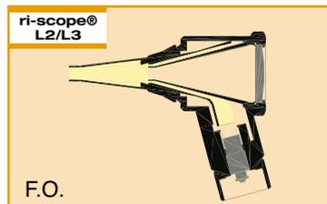
Fiber optics with 2.5-V HL halogen, 3,5-V XL xenon or 3.5-V LED illumination ensure an unhindered, glare-free view.
